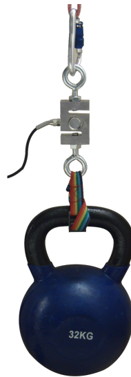
Figura 5.52: Force sensor calibration
