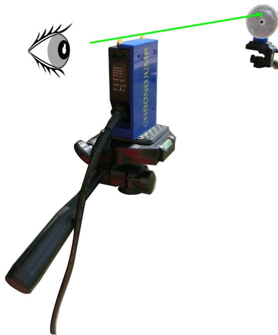
Figura 12.1: Alignment of the photocell
